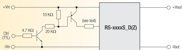
Voltage to be applied via a limiting resistor with a recommended value of 1K for RS-05xx; 3.3K for RS-12xx; RS-24xx and 10K for RS-48xx.
